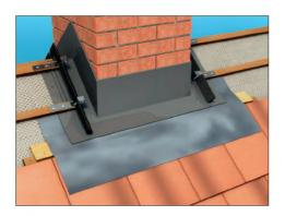
9b Fix ply section to tiling batten to create path for flashing to follow. When in situ, Dress the lead down over the tiles ensuring no ponding can occur.
