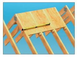
1d Check to ensure the top of the fixing support boards and top of the rafters are level.
