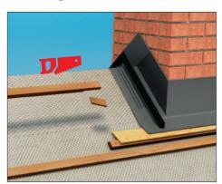
Where tiling battens meet GRP fixing flange, batten ends must be notched to ensure the batten sits flat and does not kick up.
