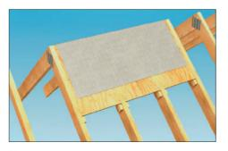
2a Install a base layer membrane over fixing support boards and secure as recommended.
