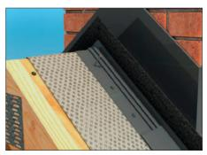
In order to secure the chimney to the support board drill 6mm holes spaced at 150mm centres along edge of GRP plinth as shown. Fix chimney to the support boards through pre-drilled holes using the recommended fixings.
