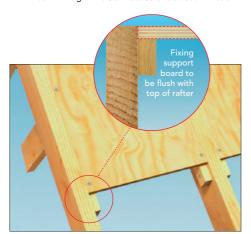
**1b** Ensure the position the battens is low enough to allow the fixing support boards to lay flush with top of the rafter when installed.
